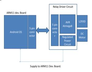
Fig. 3. Block diagram with detailed relay/motor driver circuit
