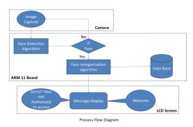
Fig.6 Process flow diagram
