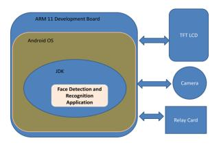
Fig. 1 System architecture block diagram
