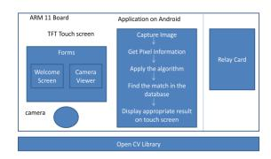
Fig. 5 System process diagram
