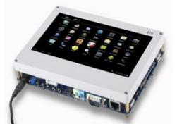
Fig.12 ARM11 dev. Board with TFT LCD
